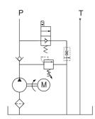
Scissor table power unit has been widely used in the industry of logistic devices such as Electric lift table, Scissor Table and Pallet Lift Table. The lowering movement is controlled by cartridge solenoid valve and its speed is controlled by the adjustable throttle valve, which can protect the Scissor table effectively. The needle release valve is used for lowering movement when the power fails to use. The manual override function is available on request.
