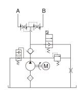
This power unit features typically power up, gravity down with machine weight function. The lowering movement is controlled by the solenoid valve while the lower speed is controlled by nonadjustable throttle valve. The high precision flow divider/combiner valve enables the synchronization of the 2 cylinders of the lift.
