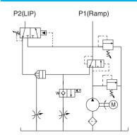
When the power pack system with a cartridge solenoid valve is normally open, it makes the ramp and lip float with the carriage during loading and unloading. The power unit also offers an emergency stop function while falling.
