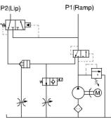
It offers an efficient and reliable control for the up and down movements of the ramp and lip of a dock leveler. Only one push button is needed for the whole operation.
