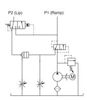
Once the power unit stops working ,the floating connection between ramp and lip can protect the oil cylinder. 60HZ motors with CSA or UL certification are available upon request.
