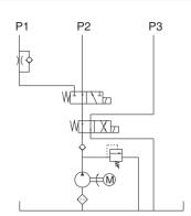
This power unit is widely used for dock leveler which need to float ramps with an emergency stop function. The ramp will rise when the pump is working. The lip will extend automatically when the ramp cylinder finishes its stroke. The ramp cylinder will retract when the pump stops running. An emergency stop will be realized while the solenoid valve is energized. The lowering speeds of both the ramp and the lip are adjusted by the throttle valves in the system.
