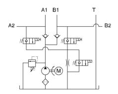
Equipped with the zero leakage double-check solenoid valves, it fulfils the complete separation of the two independent circuits which are respective for the main platform and subordinate platform of the double scissors lift. By increasing the number of the solenoid valves is easy to get more independent circuits, which are used to control the corresponding hydraulic cylinders.
