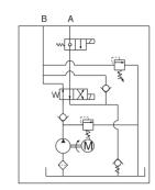
This power unit is designed solely for dump trailer, by motor power up, gravity down with vehicle weight. The second relief valve provides an extra protection for the machine when lowering. To push the start button on the motor can lift the trailer. The lowering movement is activated by the solenoid cartridge valve, while the lowering speed is controlled by cartridge flow valve in the return circuit.
