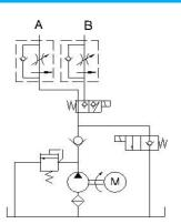
With a closed structure, this power unit is used to control the opening closing and lifting lowering of tailgates of trucks. The pressure is compensated by the flow control valve, so that can make sure to be regulated the opening and lowering speed automatically.
