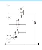
This power unit features the motor power up, gravity down with material weight. By energizing 2 position 2 way cartridge solenoid valve can lift the material and energizing the electric-hydraulic proportional valve can achieve the lowering movement.
