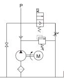
Electric pallet stacker Power Packs is designed with a two-way two-position solenoid valve to control cylinder operation. Manual control for cylinder operation is also available.
