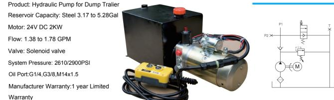
This power unit is designed solely for dump trailer, by motor power up, gravity down with vehicle weight. To push the start button on the motor can lift the trailer. The lowering movement is activated by the solenoid cartridge valve, while the lowering speed is controlled by cartridge flow valve in the return circuit.
