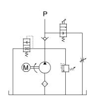
The electric-basketball Stands Power Units is designed exclusively for the electric-basketball stand, consisting of two independent, typical "power up, gravity down" circuits for the up and down movements of the basketball board and the whole basketball stand. The pressure switch will stop the motor once the basketball or the whole stand is compensated by the balance valves which make the lowering movements very smooth.
